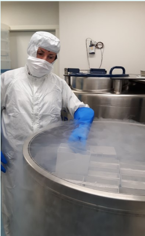
Joy Buckley at Nitrogen tank with stem cell bags in storage.
